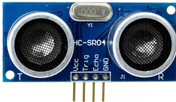
Figure 24. HC-SR04 Ultrasonic Sensor
